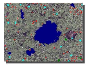
Objects can then be automatically classified into groups of objects with similar measurement characteristics or, as in this case, classified according to measurement intervals defined by the user. Here the user has created four classes of objects based upon specific area criteria. For example, there are five objects in the largest area class, shown in blue on the image and in the data table.
