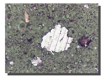
After use, metal lubrication fluids contain bits of metal called "wear metal". The efficiency of a lubricant and its effects on machinery can be measured by the amount of wear metal (bright particles in the image) found in the lubricant after a certain period of usage. The less wear metal found in the lubrication, the better the lubrication is performing. The results of microanalysis are used to make recommendations taking into account the age of the equipment, the type of lubrication used, etc.
